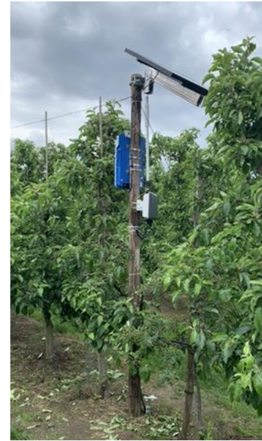
Each sensor wirelessly sends data to centralized 5G router in the orchard, which transmits continual data via cellular network
