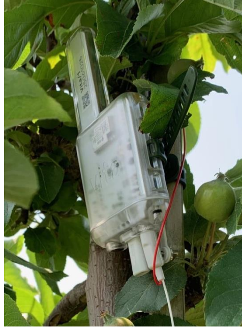
Sensors are installed directly into the trees. 32 Trees and 64 sensors.
