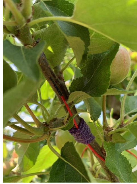
Electrodes are connected to the sensors and inserted to tree branch vasculature
