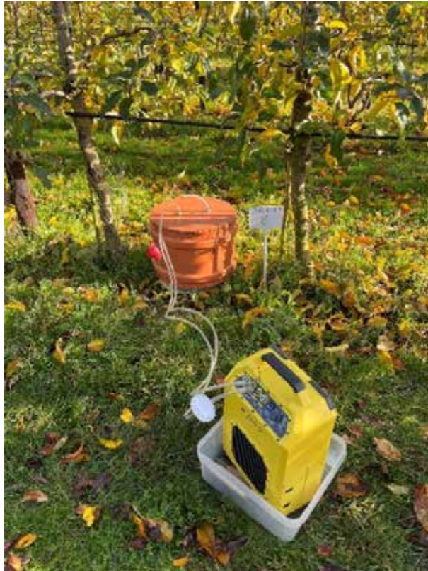
Picture 10. Cranfield's in-field greenhouse gas emission monitoring equipment in orchards.
