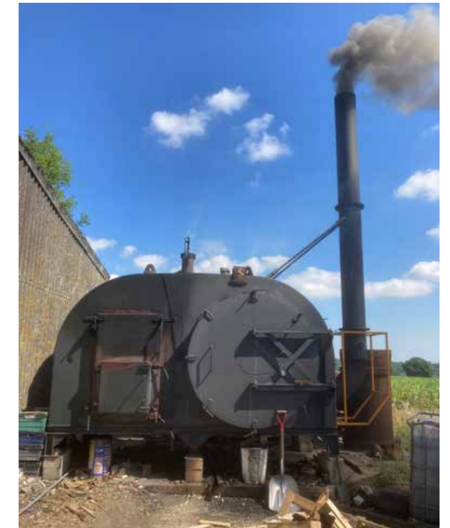
Picture 4. Ashdown Logs and Charcoal's Pressvess batch kiln.
